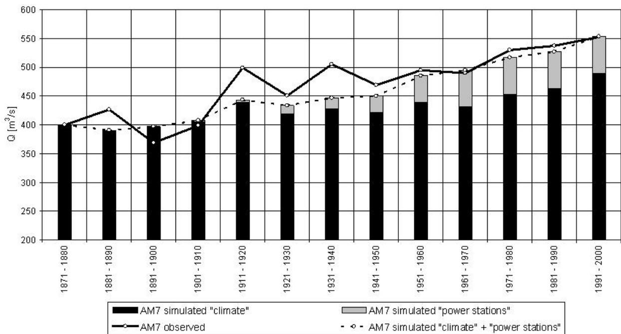
**Fig. 5** Rhine at Basel: observed and simulated  $AM_7$  values (10-year means) from 1871 to 2000. The effects of Alpine reservoirs and climate change can clearly be distinguished in the simulation.
