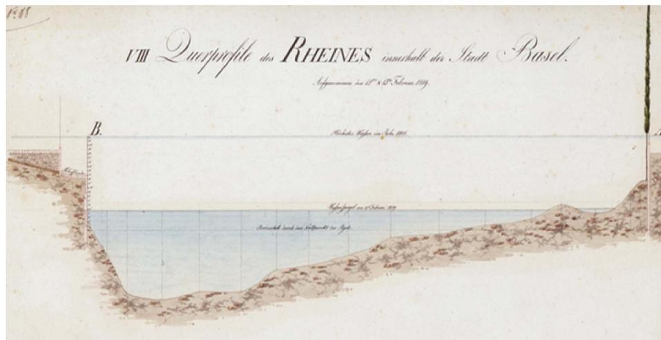
Fig. 5 Cross-section of the Rhine at Basel, drawn on 15 February 1819 (Source S1).
