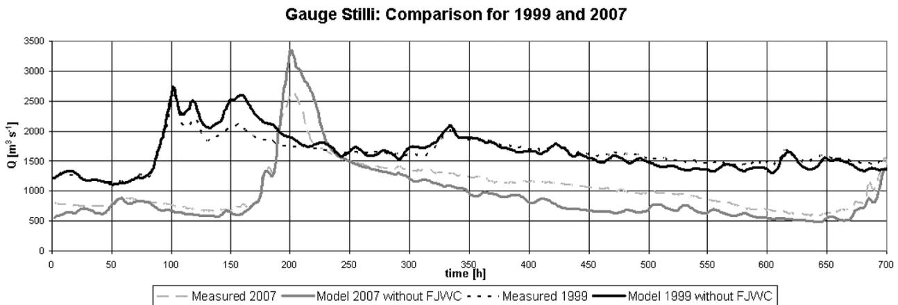
**Fig. 13** Observed (including first Jura-Waters Corrections FJWC) and simulated (situation prior to 1868, i.e. without FJWC) flood hydrograph of the 1999 and 2007 flood events for the River Aare at Stilli.
