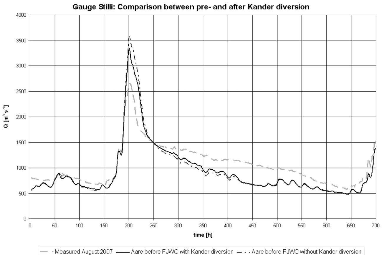
**Fig. 14** Observed and simulated hydrographs for the River Aare at Stilli: simulated effects on peak discharge of the River Aare on the supposition of pre-Kander (1714) and pre-Aare (1877) diversions.
