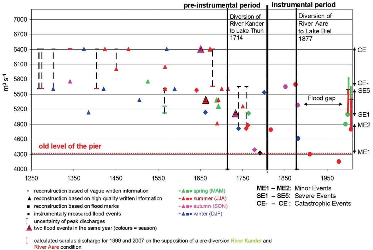
**Fig. 9** Rhine River discharge quantities 1250–2010; calculations based on documentary and instrumental evidence (peak discharge values are given as they were observed; no adjustment to either pre- or post-Kander/Aare diversions was made).
