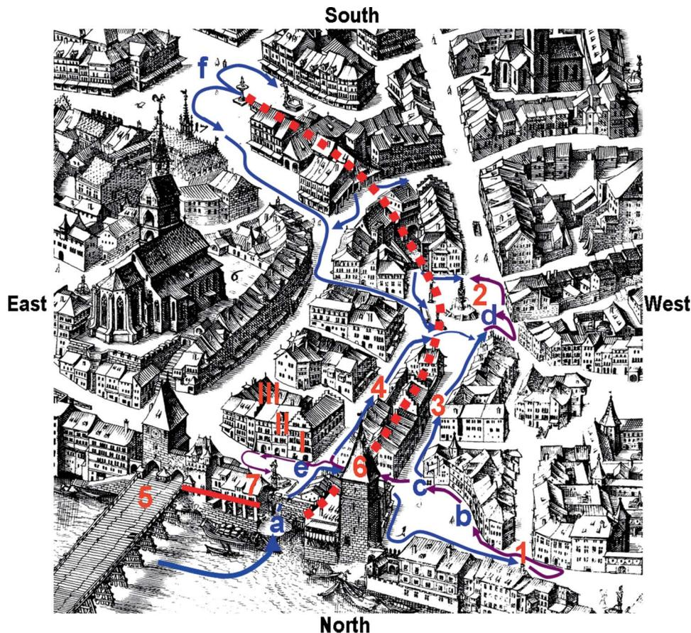
**Fig. 4** Bird's-eye view by Matthäus Merian, 1615 (Source S20). Blue arrows indicate the direction of water flow; purple arrows – water accumulation; red bar: approx. the same height of the bridge and the windows of the Guildhouse; and red dotted line: underground flow of Birsig brook.
